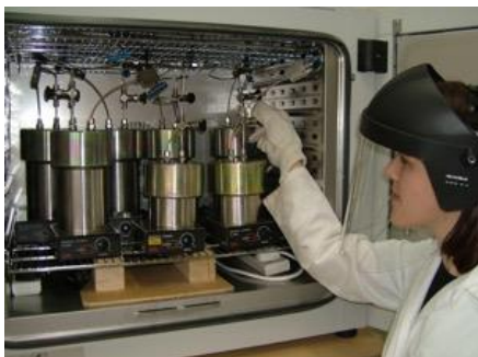
Laboratory capability at the British Geological Survey allows rock samples to be exposed to hydrogen at 50 degrees Celsius and 150 bars of pressure- conditions approaching those where hydrogen could be stored underground
